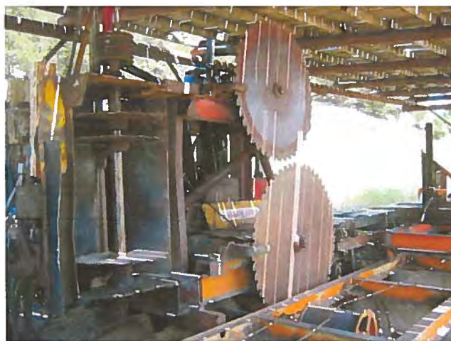
Detail of Sawmill with top saw and vertical edger
